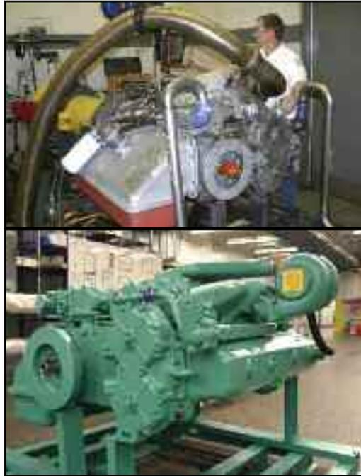
***(top) JASPER Associate Brian Seger puts the 6-71TA 'pancake engine' through its paces on the dynamometer. (above) The finished engine, ready for work.***
