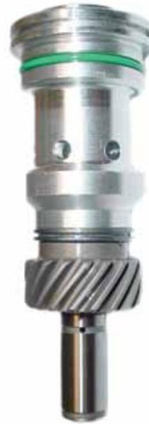
***The next time you replace a Ford 4.0L OHC V6, be sure you grab the oil pump intermediate drive from the core engine.***
