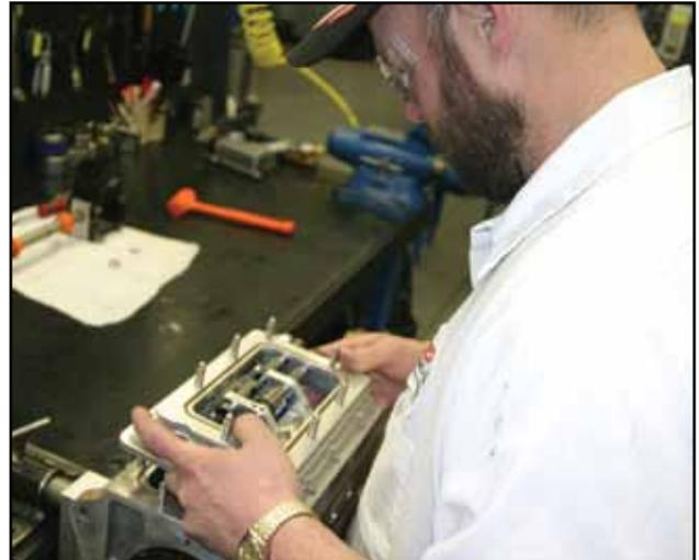
***Associate Danny Berry attaches the shift body of the JASPER 4-Speed Single-Rail to the case.***
