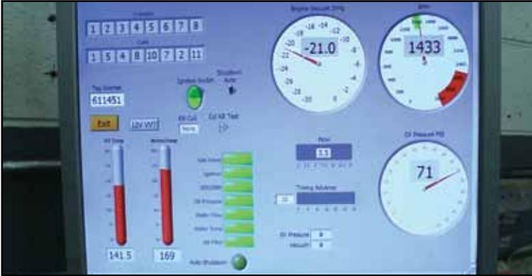
**Once oil temperature reaches 145 degrees, the data acquisition system takes a snapshot of the engine readings displayed.**
