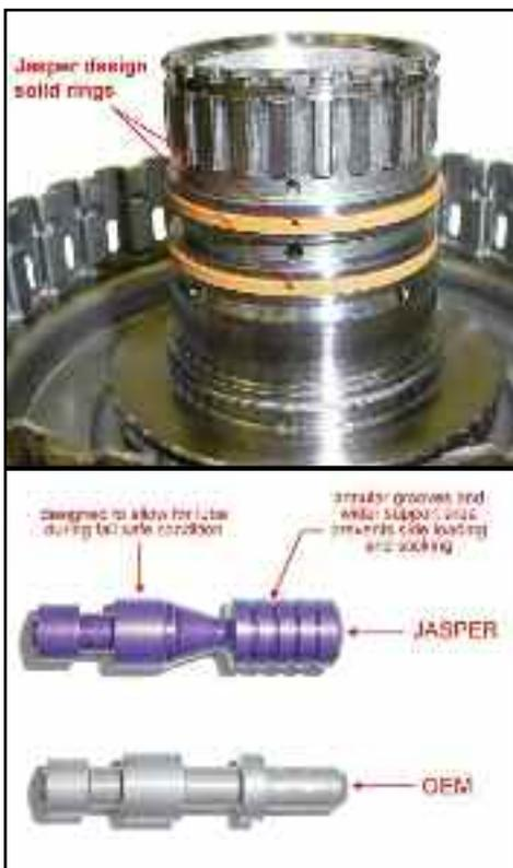
**(Top) Solid rings are used in the forward drum of the CD4E in place of scarf-cut rings. (Above) The converter regulator used in the JASPER CD4E compared to the OEM design.**
