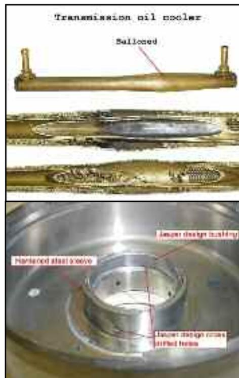
**(Top) OEM coolers have been found to fail internally and restrict cooler flow. (Above) JASPER redesigns the CD4E reverse drum to be more durable and supply direct lubrication to the bushing journals.**
