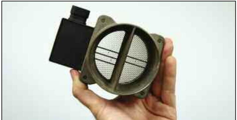
**The Mass Air Flow, or MAF, sensor. This one comes from the intake of a GM Vortec V8.**
