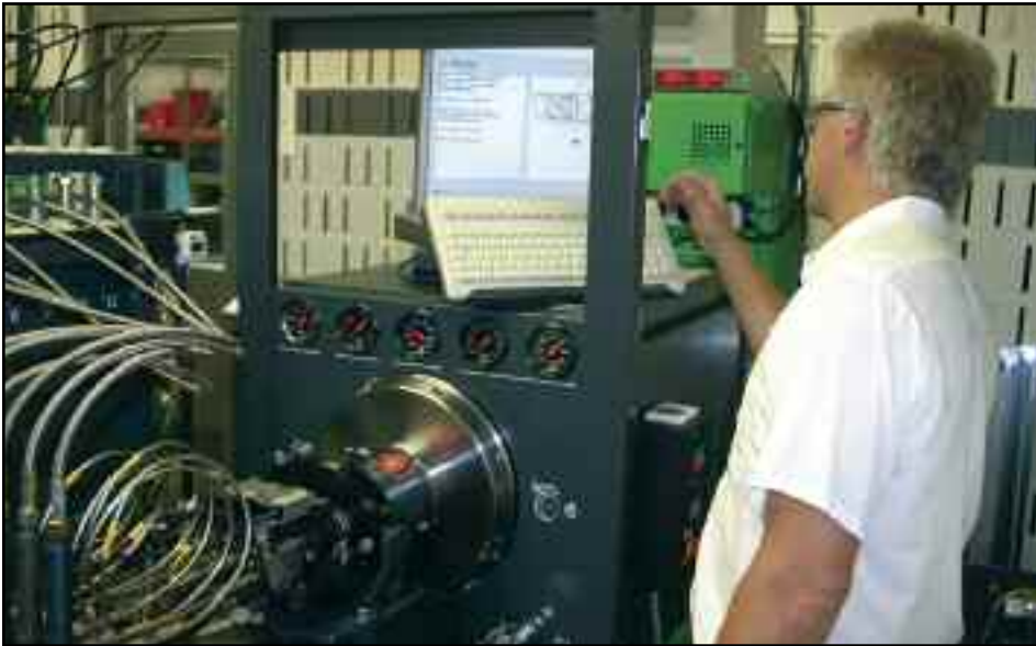
JASPER Fuel Room Associate Ron Hornaday prepares a Bosch VP44 pump for testing on the new EPS 815 computerized test stand.
