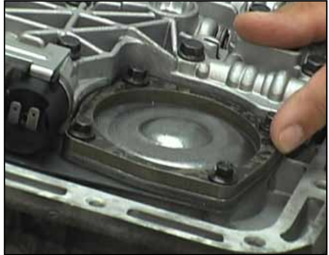
This support plate, mounted over the reverse servo cover of the Ford 4R55E/5R55E, allows the transmission to maintain reverse in 1995-2008 Ranger, Explorer and Aerostar.
