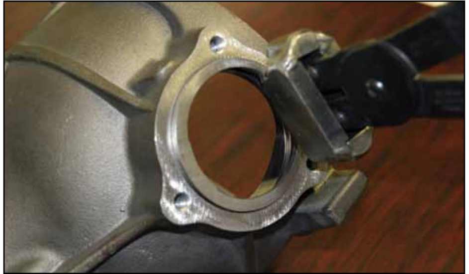
Figure 1: It takes a modified pair of retaining clip pliers to compress the .174 thick ring for installation into the Jeep Grand Cherokee front differential. JASPER stocks 98 different-sized snap rings of varying thicknesses in .001 increments.
