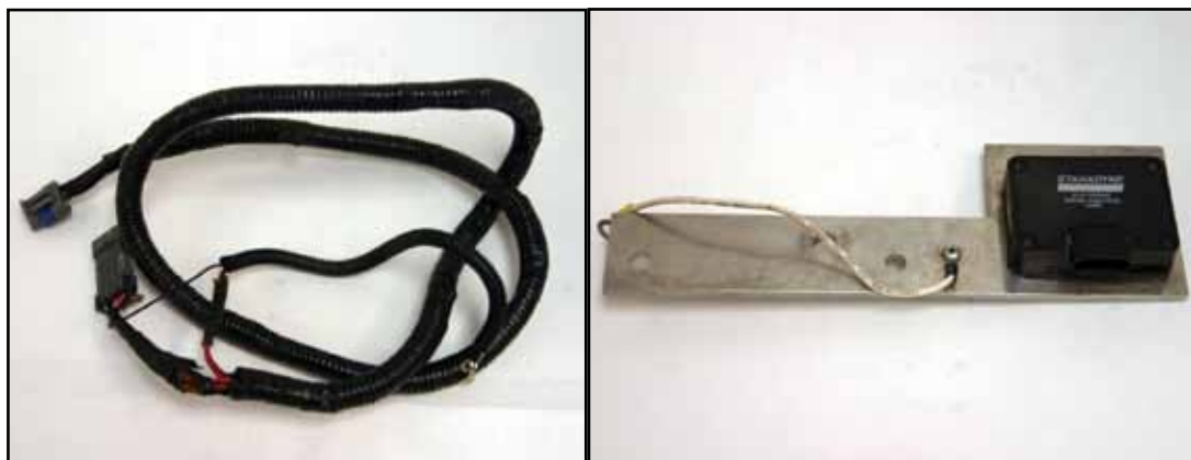
(Above left) Relocating the PMD could cause circuit-related issues as the wiring harness is extended, spliced into or stretched. (Above right) Aftermarket heat exchangers are not beneficial to the life of the PMD or the reliability of the injection pump as a whole.
