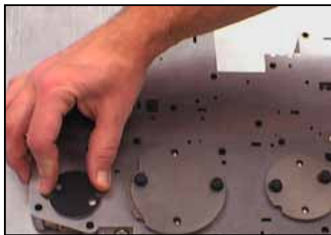
This is the location JASPER will drill and tap to accommodate the reinforcement plate, reducing the possibility of gasket failure.
