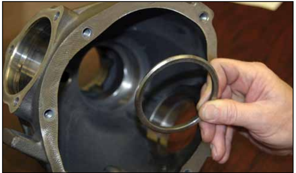
Figure 2: This pinion depth shim measures .213 thick. JASPER keeps 75 different-sized pinion depth shims of varying thicknesses in .001 increments.
