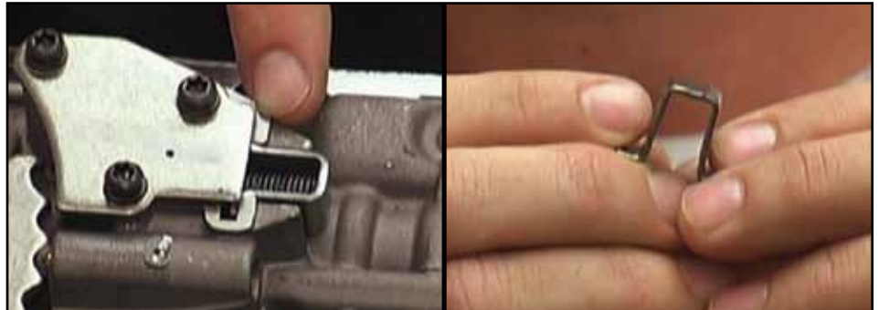
(Above left) This little clip holds the boost valve spring in place on the valve body. (Above right) The clip is made of stamped steel and will break at one of the weak bend points.
