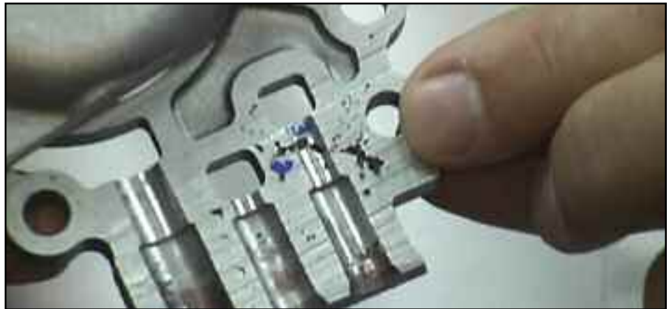
These pores were found in the aluminum accumulator housing of a GM front-wheel drive transmission. These pores caused the part to fail JASPER's transmission circuit test.
