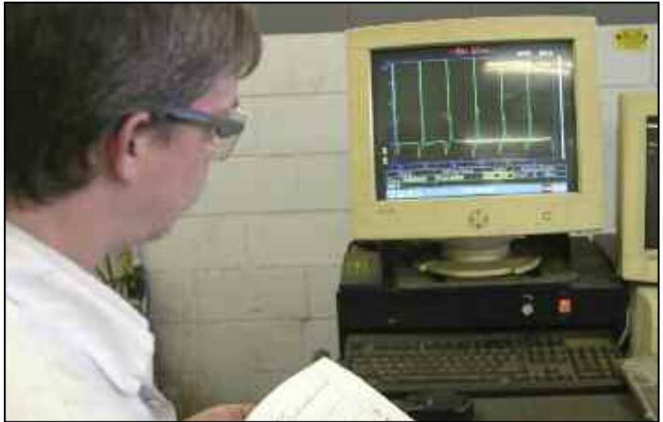
Comparing your labscope findings against a known waveform for a particular circuit could be your best way to determine internal engine issues.
