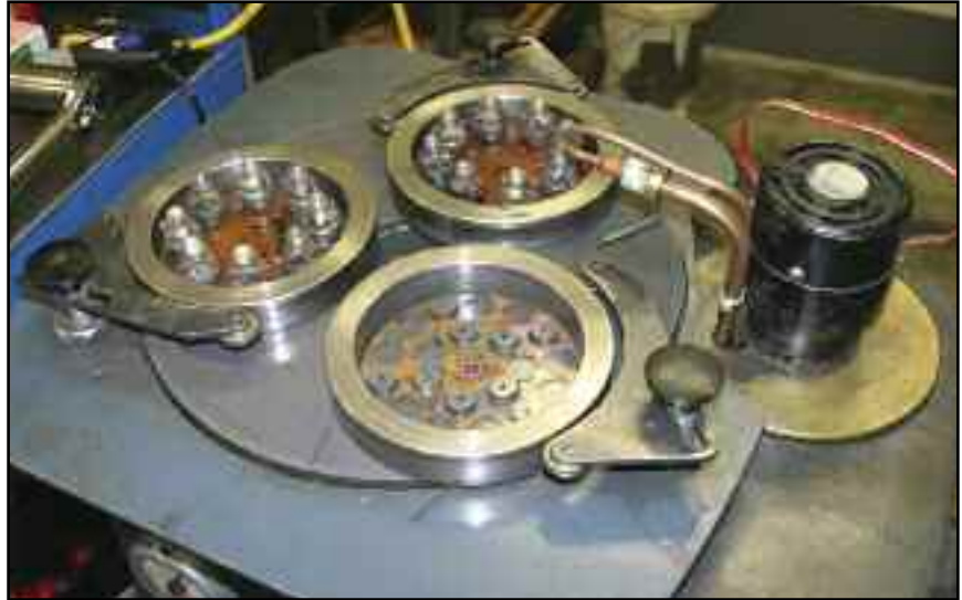
Each injector body and intermediate disk of the GM 6.5L TE Running Complete is lapped on a lapping machine to help eliminate any type of warpage and safeguard against leaks.
