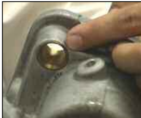
Figure 1 - A brass bushing is driven into the RWD Chrysler overdrive transmission case.
