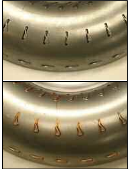
This is what the outside of the 4L80E turbine half looks like before (top) and after (bottom) the JASPER update.
