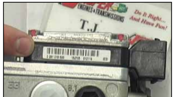
JASPER verifies the date code on the PSG, and reflash-es the electronic controller, eliminating limited key cycle concerns.
