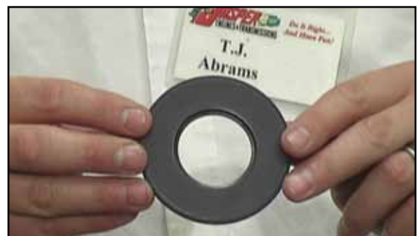
A thicker, metal-plated diaphragm is installed to help eliminate low fuel pressure problems within the pump.
