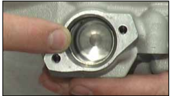
JASPER uses steel inserts in the advance cylinder bore in place of the original brass insert, eliminating severe wear issues.
