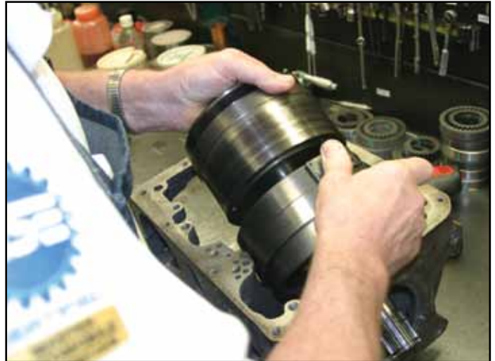
The clutch packs of the Hydramatic are fitted inside the case during final assembly. This transmission came from a 1956 Oldsmobile Rocket 88.
