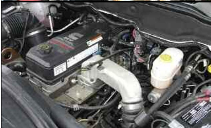
**Top: Cummins 6BT engine from 1991 Dodge Ram 250. Above: Cummins ISB engine from 2007 Dodge Ram 3500. JASPER has both engines available either as a Complete or Running Complete engine.**
