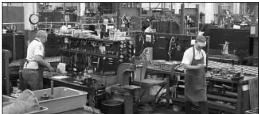
**The new trunk line in Transmission Assembly delivers prepared transmissions directly to assembly teams, then delivers the unit to the test room.**
