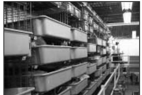
**A 58' long computerized carousel holds up to 88 transmissions ready for final assembly.**
