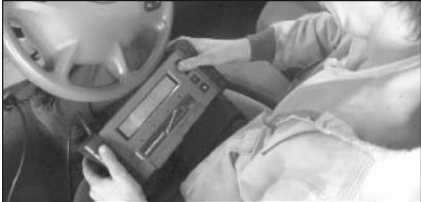
**When you diagnose a hard shift complaint, monitor what the computer is seeing. You can determine if the complaint is the cause, or the result, of the problem.**
