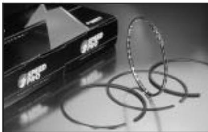
The race proven open gap design intentionally allows an escape path for residual combustion gases, reducing inter-ring pressure and keeping the top ring sealed against its groove. Without this escape path, trapped pressure will unseat the top ring, causing ring flutter and reduced cylinder seating at high RPM. One piece second rings are far more effective and reliable to retain combustible pressure lost through ineffective top rings. Beware - cylinder leakage tests are steady state - they
