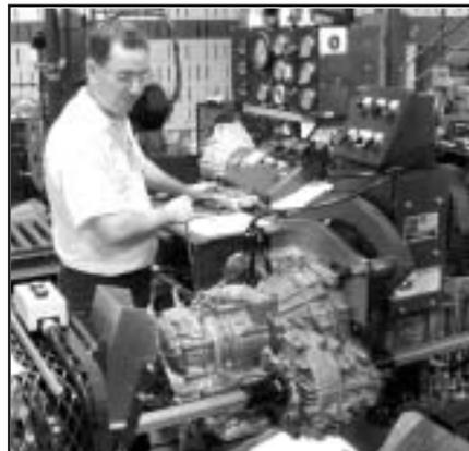
**JASPER associate Keith Songer tests the Toyota A541E on the dynamometer.**
