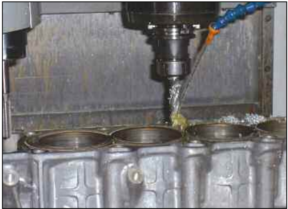
The CNC-controlled boring machine conducts the 20 head bolt hole repairs and 20 main bolt hole repairs on the Cadillac 4.6L Northstar aluminum block.
