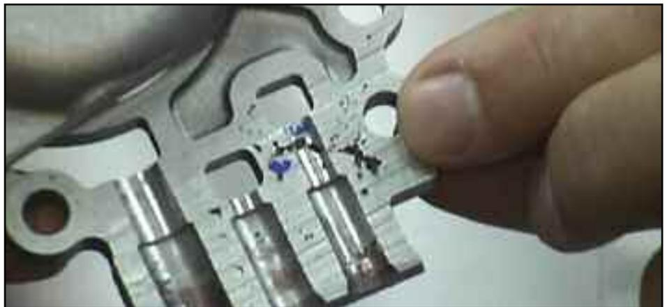
**These pores were found in the aluminum accumulator housing of a GM front-wheel drive transmission. These pores caused the part to fail JASPER's transmission circuit test.**
