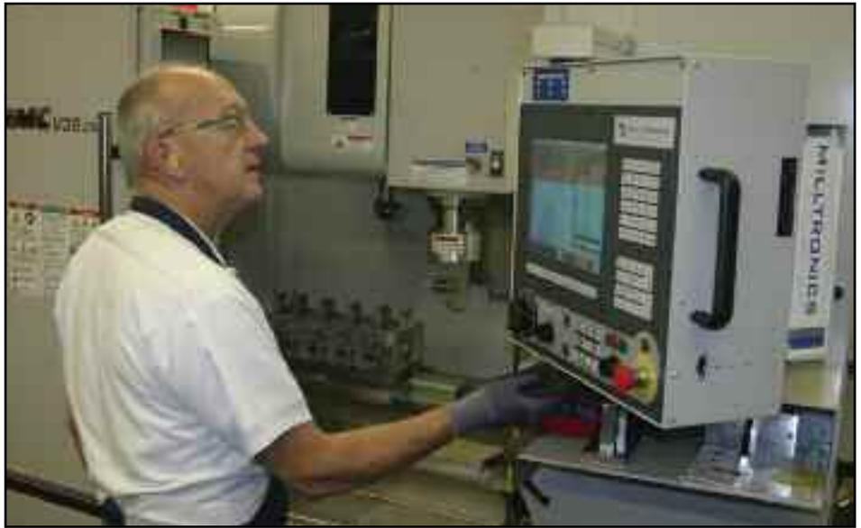
**JASPER Associate Dave Loechte prepares a Ford 4.6L modular cylinder head for cam bore alignment on the Milltronics 7200 CNC machine.**
