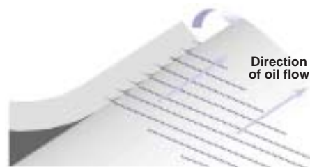
Figure 2 - The PTFE sealing element acts like a pump.
