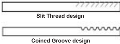
Figure 3 - Alternative PTFE element designs.
