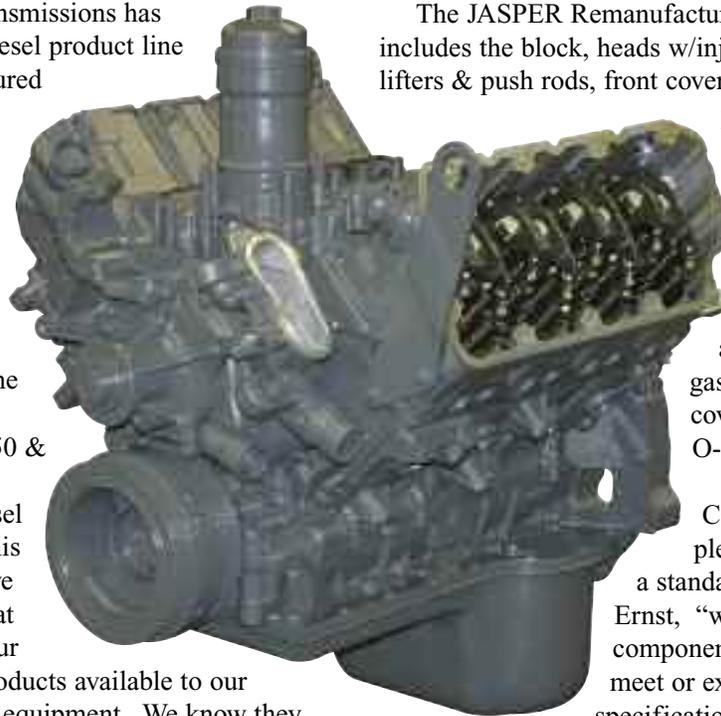
The JASPER Remanufactured 6.4L Complete engine includes the block, heads w/injector tubes, crank, cam, lifters & push rods, front cover, vibration damper, water pump, oil pump and pan, new oil cooler, oil filter assembly, new head bolts, rear cover, front & rear seals, lower rocker housing and rocker assemblies. The engine also includes valve cover gaskets, breather to valve cover gaskets and a dipstick O-ring.
