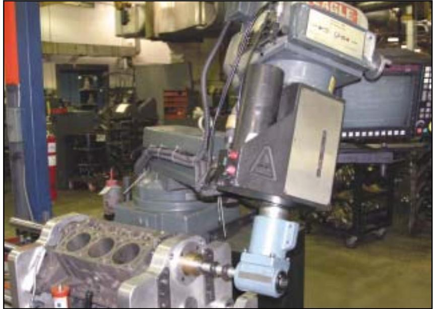
**The CNC-controlled align boring machine eliminates cam bore alignment issues on the GM V6 engine before bearings are installed.**
