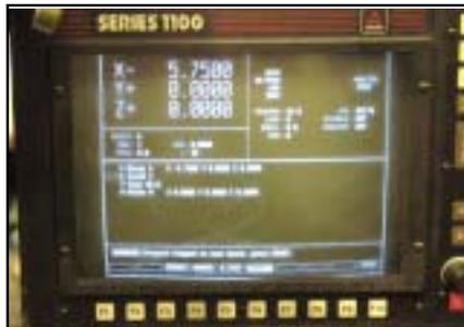
**The CNC computer keeps track of the align boring process.**
