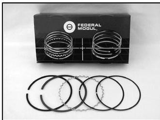
One final point on ring end gaps: Some engine builders are reluctant to use standard end gaps with hypereutectic pistons due to limited problems associated with ring land breakage. This problem is a function not of the piston ring or piston material but the manufacturer's piston production process. In manufacturing hypereutectic pistons, it's
