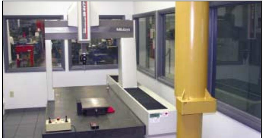
*It has its own room: JASPER utilizes this Coordinated Measuring Machine to verify new internal components, major castings or assist in the reverse engineering of components.*
