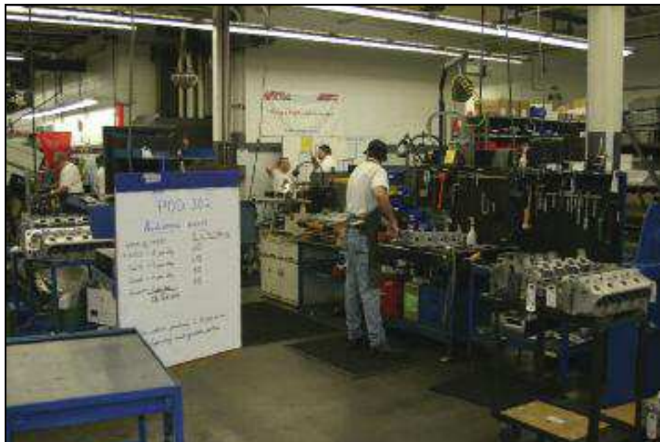
Each pod in the Gas Engine Department has the machinery and tools necessary for block and head remanufacturing.
