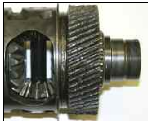
Figure 2 - That metal tab from the washer had to go somewhere... and eventually destroyed the case gears.
