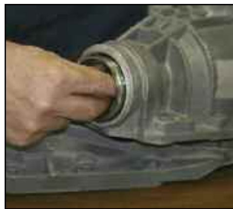
Figure 2 - JASPER will use retaining compound to keep the outer pinion bearing from spinning within the aluminum housing.
