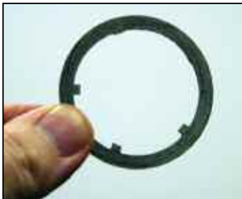
Figure 1 - The washer hidden underneath the final drive sun gear of the 4T65E gearbox has one worn tab and one tab missing.
