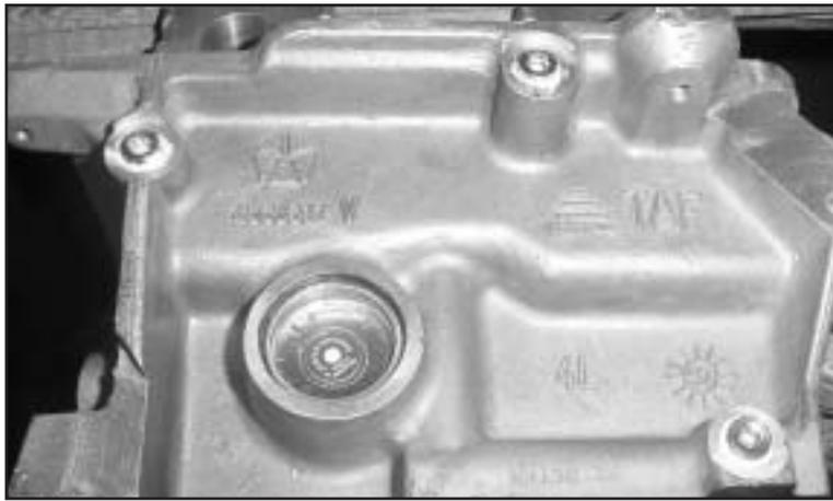
**JASPER drills, taps and plugs the Chrysler 2.7 liter heads to eliminate the chance of oil leaks.**
