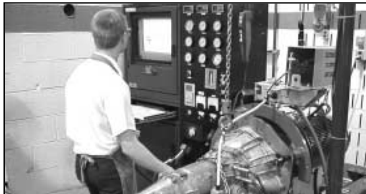
One of the first dynamometers JASPER designed to test transmissions (pictured at top) is still in use for older hydraulic transmissions. In JASPER's newest dynamometer (pictured above), the computer controls today's electronic transmissions per a set program.
