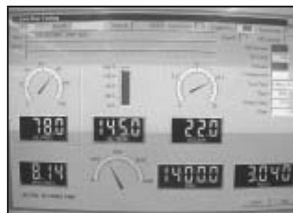
**Engine oil temp and pressure, oil flow, water temp and vacuum is recorded.**
