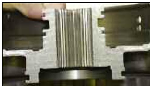
**JASPER ensures these 4R100 transmissions have a full spline engagement of the input shaft.**
