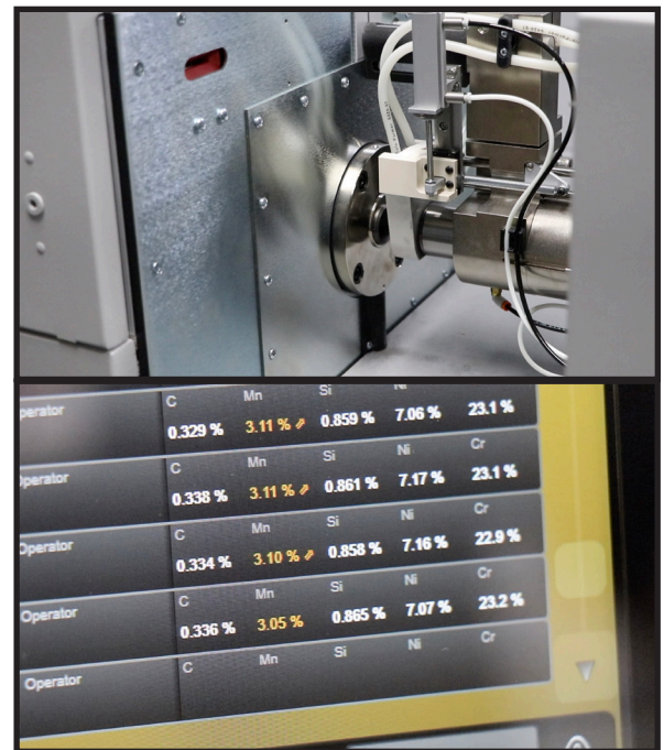
The LECO Mass Spectrometer burns a sample from a metal-alloy component (top), in this case an intake valve. The machine evaluates the ions from the sample burn revealing the chemical composition of that alloy (above).
