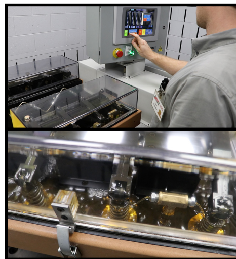
The Ahaus Valve Stem Seal Tester (top) measures how much oil flows past a valve seal. Seals are tested under pressure and vacuum (above) at engine operating temperatures and at various speeds.
