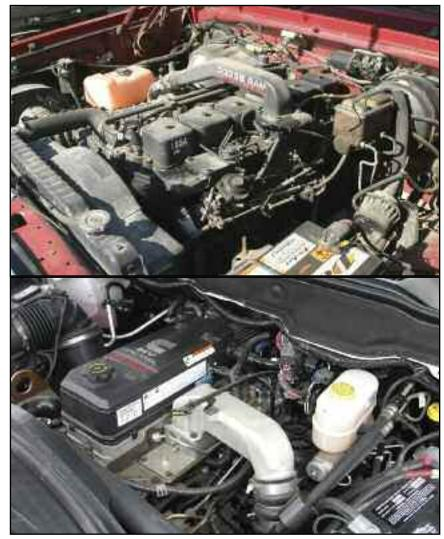
Top: Cummins 6BT engine from 1991 Dodge Ram 250. Above: Cummins ISB engine from 2007 Dodge Ram 3500. JASPER has both engines available either as a Complete or Running Complete engine.
