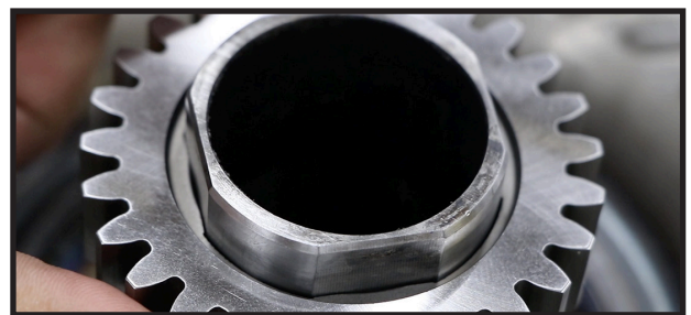
The beveled pump gear reduces the amount of play the gear has with the impeller hub, ensuring consistent fluid pressure.
