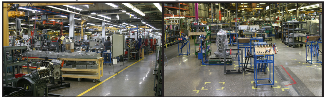
POD 70 of the Diesel Division (left) remanufactures the current lineup of V8-style engines, including the 6.0L, 6.4L, 444 and Duramax engines. POD 90 (right) is in the initial setup stages, and will remanufacture several of the popular inline diesel engines from Cummins and Caterpillar.
