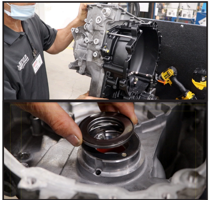
(top) JASPER designed a 6F35 case template to machine worn aluminum surfaces of the axle drive sprocket. (bottom) A steel pad is installed on the case for the thrust bearing to ride against.
