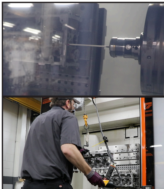
A Renishaw probe (top) identifies the head inside the Mazak CNC unit, assigning the proper machining operation. The tombstone (bottom) can hold up to four cylinder heads.
