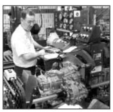
JASPER associate Keith Songer tests the Toyota A541E on the dynamometer.
