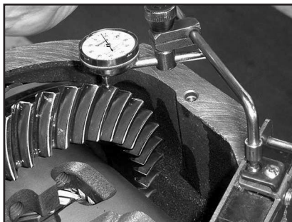
This is the proper way to measure pinion-to-ring-gear backlash.
