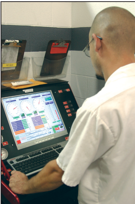
JASPER Associate Heath Eckerle pours over the numbers while the diesel engine undergoes dynamometer testing.
