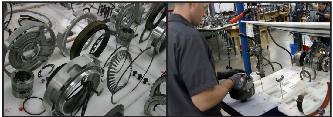
(Above left) Every transmission part has a specific place on a board, so Associates can quickly see if they have everything for assembly. (Above right) Associate Chris Hemmer facilitates 'one touch assembly' which reduces overall parts handling within the work area.
