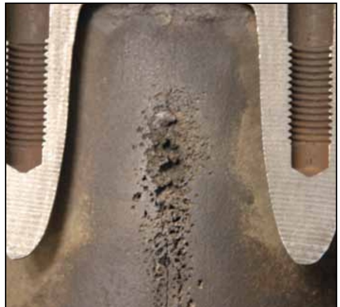
Figure 1 - This cutaway of an International 7.3L diesel block shows cavitation present on the outside cylinder walls.
