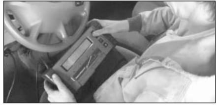
When you diagnose a hard shift complaint, monitor what the computer is seeing. You can determine if the complaint is the cause, or the result, of the problem.
