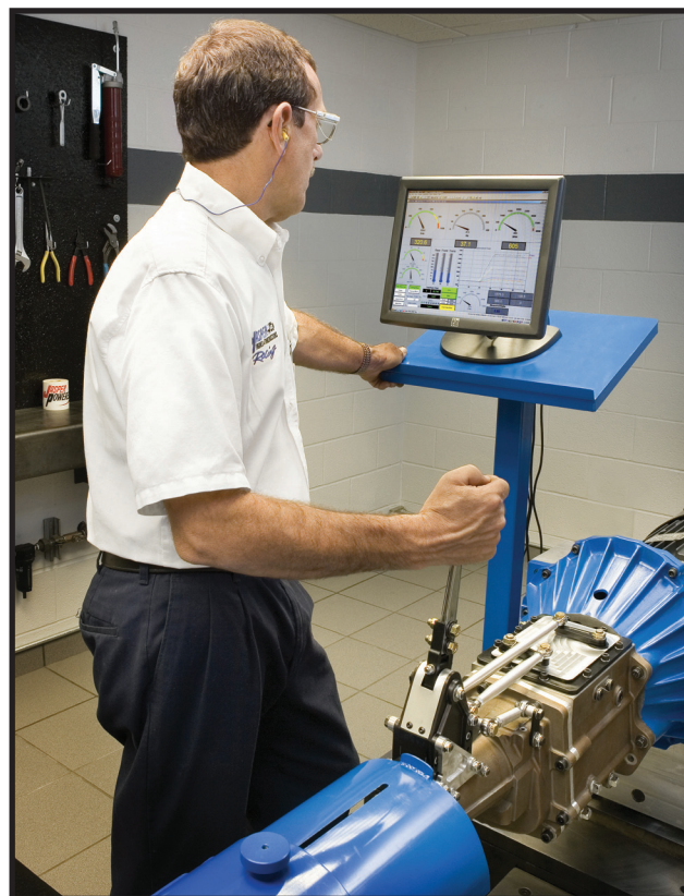
Driveline Division Manager, Terry DeKemper, tests a JASPER traditional three-rail 4-Speed Transmission.
