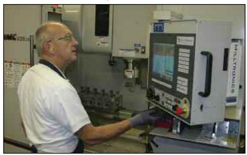
JASPER Associate Dave Loechte prepares a Ford 4.6L modular cylinder head for cam bore alignment on the Milltronics 7200 CNC machine.
