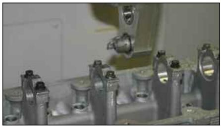
The cutting head on the Milltronics 7200 CNC machine is in the middle of align boring a Ford 4.6L modular cylinder head.
