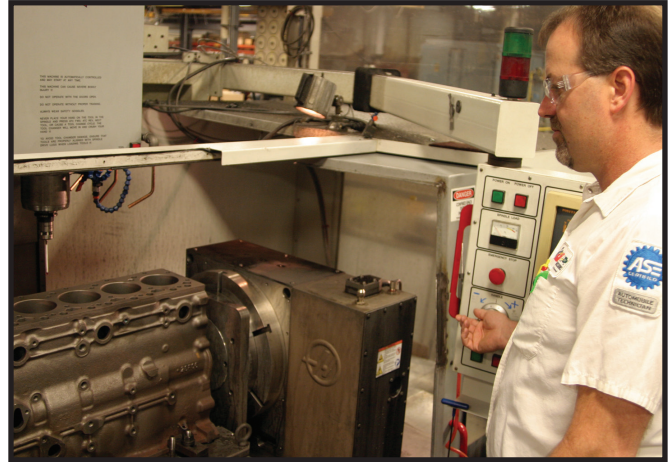
Jonas Cox, JASPER Diesel Associate, prepares a Cummins engine block for honing and boring using the Haas VF-6 CNC machine. JASPER has numerous CNC machines within various departments. This is the latest machine to arrive within the Diesel Division.
