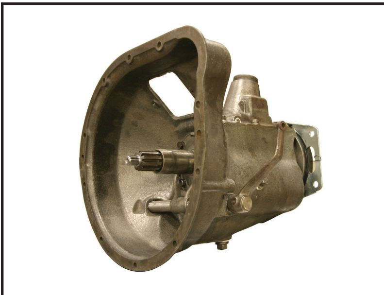
This three-speed manual transmission from a 1932 Ford Model B was recently remanufactured by Jasper Authentic Custom Drivetrains.
