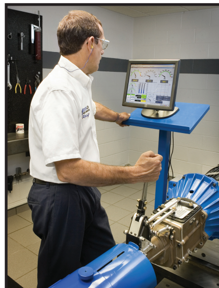
Division Manager Terry DeKemper tests a JASPER traditional three-rail 4-Speed Transmission.
