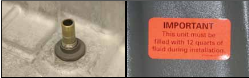
Figure 1 (above left): Inside the pan of the 5R55N/S/W is a tube which determines the transmission fluid level. Figure 2 (above right): A sticker reminds technicians the transmission holds 12 quarts of fluid.
