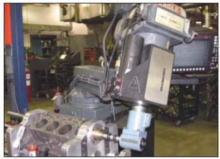
The CNC-controlled align boring machine eliminates cam bore alignment issues on the GM V6 engine before bearings are installed.
