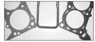
Left to Right: Fiber paper steel head gasket; cork valve cover gasket; multi-layer steel gasket.
