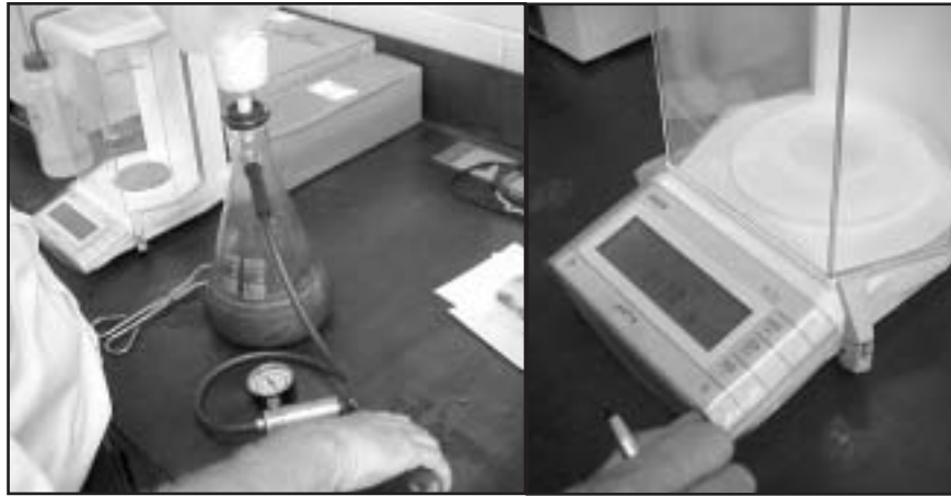
Residual particles collected in solution are filtered through 20 micron filter paper, then dried to record sediment weight.
