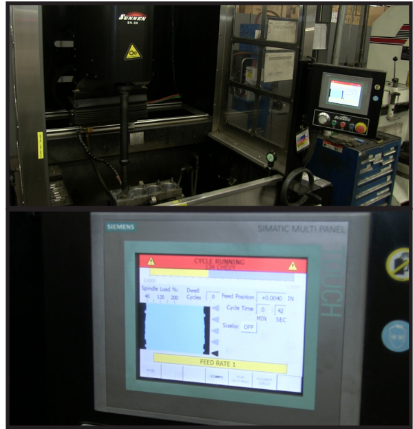
The Sunnen SV20 uses automated size control, and recall memory, so that all cylinders in a particular block can be honed to the exact same spec.
