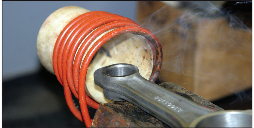
The induction heating coil, coupled with an electronic timer, is used to assemble connecting rods with a more accurate control on the heat.
