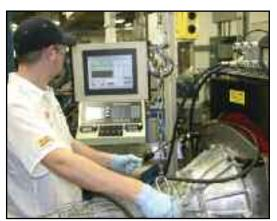
In With The New - JASPER Associate Aaron Schipp puts the new Axi-Line computer controlled electric dynamometer through its paces.
