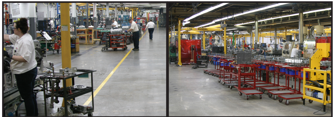
Associates in new Gas Engine Division work areas (left) have more room to operate, and open aisle ways allow for easier material flow. The new work area configurations, highlighted by yellow overhead hoists (right), slowly overtake the older-style Gas POD layouts.
